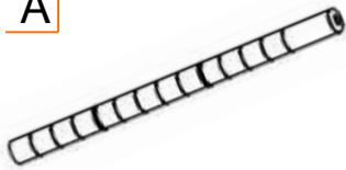
BOTTOM POLE (4) Threaded Insert (4) is pre-installed
